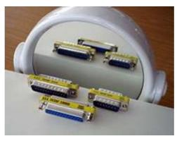
Figure 04: A Gender changer is a little piece of hardware that changes the 'sex of a computer cable'. Image of the hardware sourced at http://en.wikipedia.org/wiki/Gender\_changer
