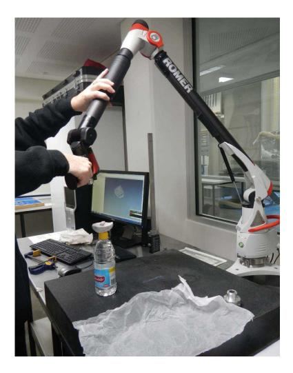
Figure 1 Potato Scanning, (2013), *ECU Engineering Department*, using a Romer Absolute Arm with an integrated scanner, Photographer Courtesy of the Artist.
